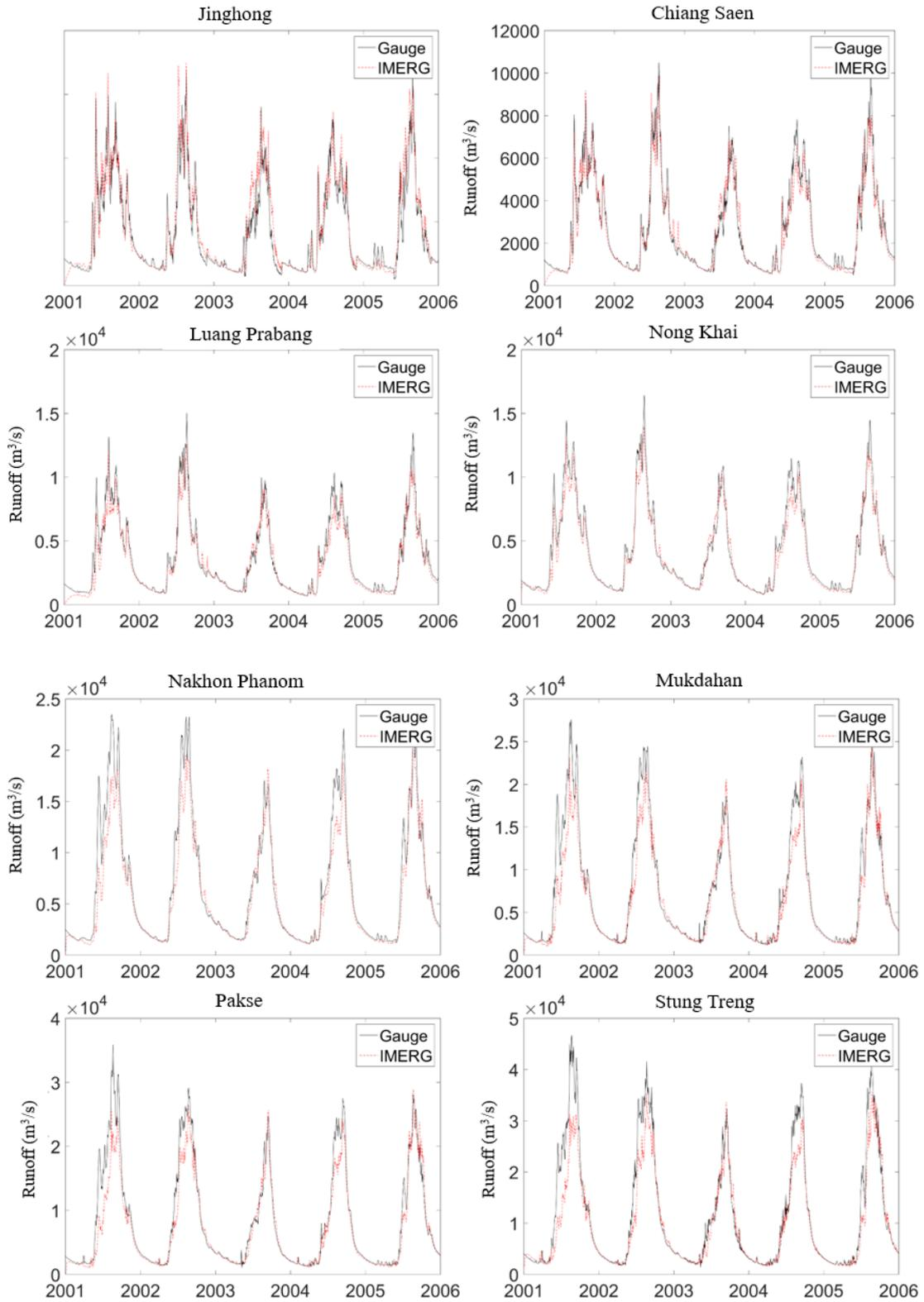
Figure 4. Streamflow simulation driven by the satellite rainfall and the gauge rainfall at 8 hydrological stations along the mainstream of Lancang-Mekong River
