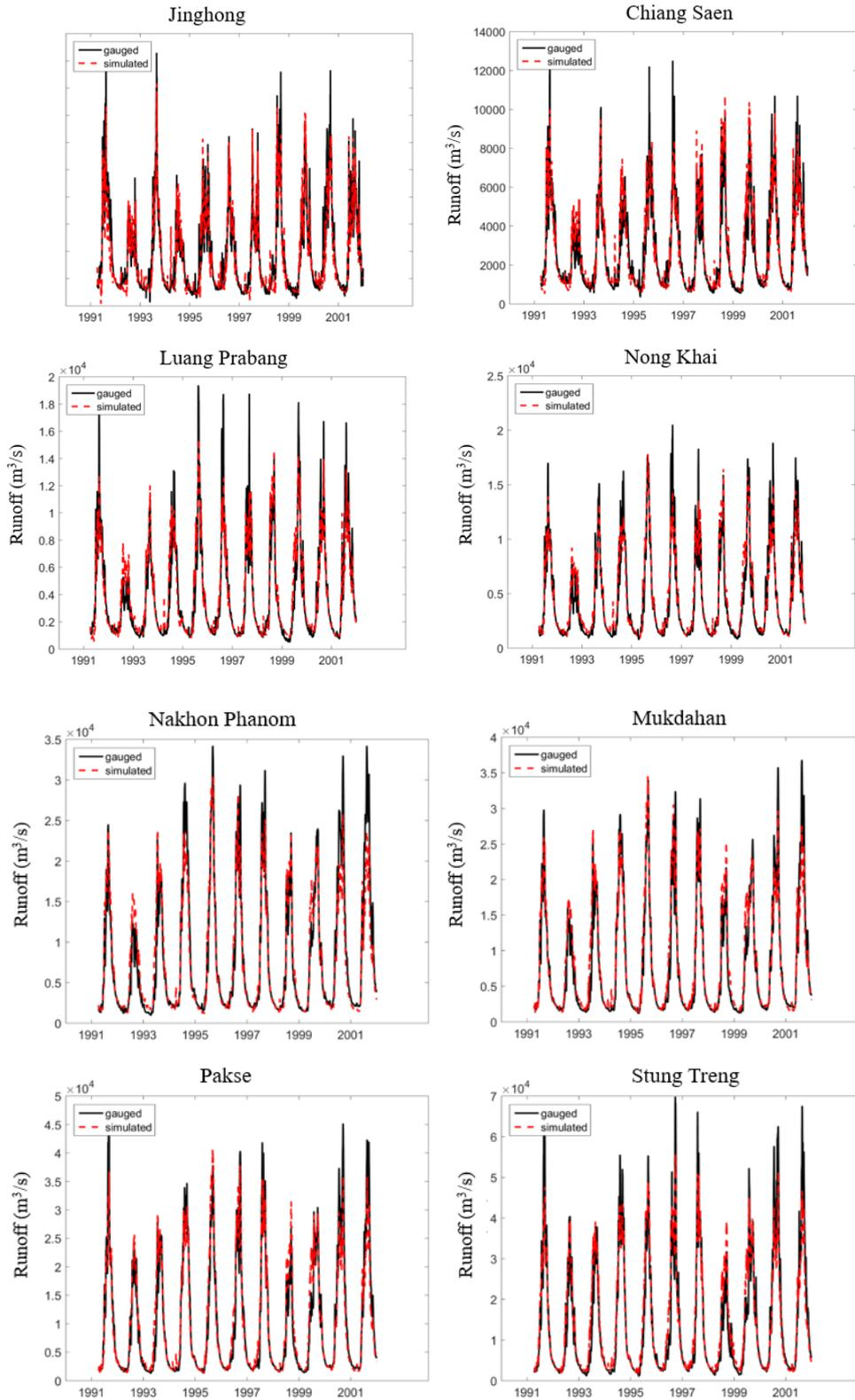
Figure 3. Simulated and observed daily streamflow at the 8 stations along the mainstream of the Lancang-Mekong River
